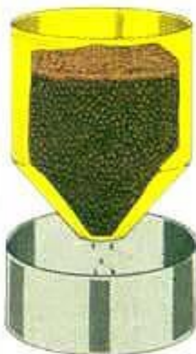
FIGURE 17. The larger the soil particle size, the lower the water-holding capacity. (a) A relatively small amount of water is held by coarse-textured soil as compared to (b) the amount held by fine-textured soil.
