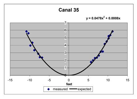
Figure 8. Cross-section of canal 35
