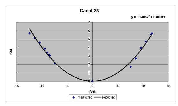
Figure 4. Cross-section of canal 23.
