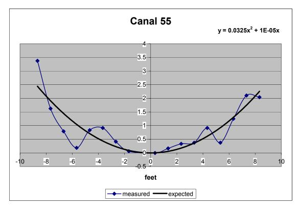
Figure 10. Cross-section of canal 55
