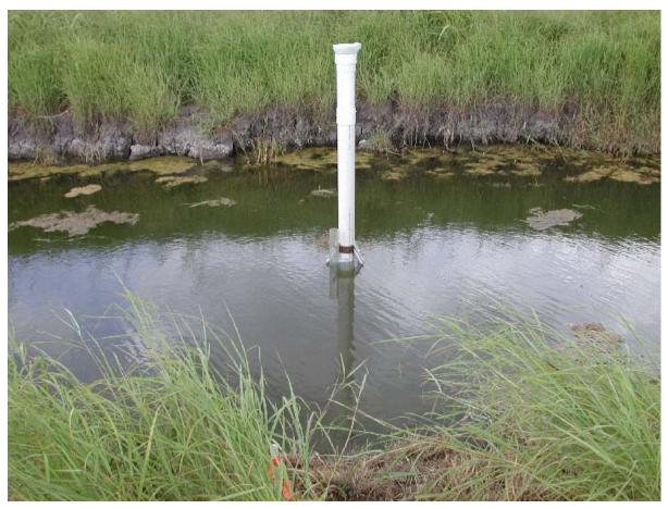
Figure 2. Continuous-stage level recorders on canal 55.
