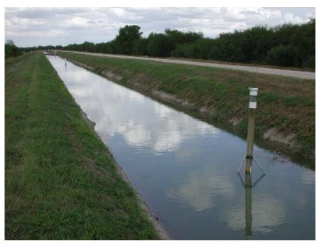
Figure 10: Continuous stage level recorders on Lateral A – "I" Rd.
