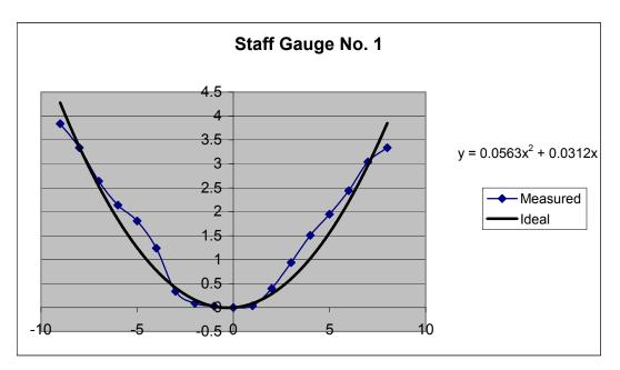
Figure 6. Cross-section of Staff Gauge 1 of lateral A - Stewart Rd.
