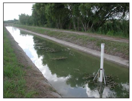
Figure 2. Continuous-stage level recorders on lateral A - Stewart Rd.
