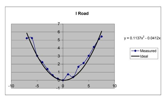
Figure 11: Lateral A - I Rd cross-section
