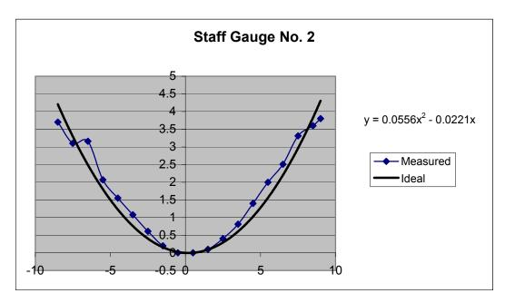
Figure 7. Cross-section of Staff Gauge 2 of lateral A - Stewart Rd.
