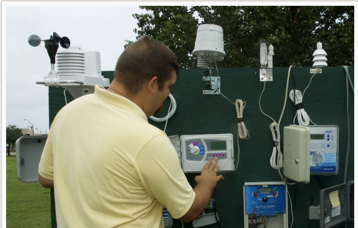
Charles Swanson, Texas AgriLife Extension Service landscape irrigation specialist, opens the programming unit of a ‘smart’ irrigation controller. Some of the different weather sensors manufacturers use on their controllers are mounted on top of the panel. (Texas AgriLife Extension Service photo by Robert Burns)
