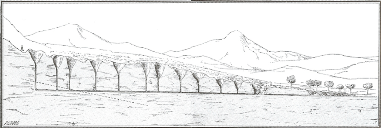
Figure 1. Diagram of a typical Afghan karez (source: Watershed Atlas of Afghanistan, UNFAO, 2004.)
