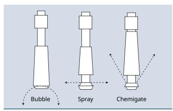
Figure 10. Original multi-functional LEPA head.
