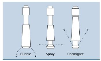
Figure 10. Original multi-functional LEPA head.
