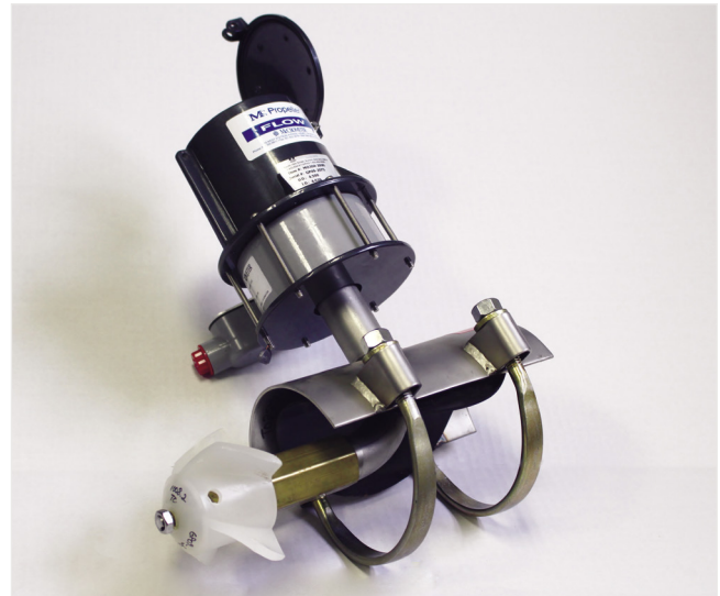
Figure 8. Saddle flow meter, which can be installed into an existing pipeline by cutting a hole in the top of the pipe. Meter shown has an optional digital output for use with irrigation control and monitoring systems.
