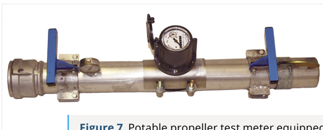
Figure 7. Potable propeller test meter equipped with a pressure gage, quick-connects, and handles for insertion into existing water supply pipelines for measuring flow rates.
